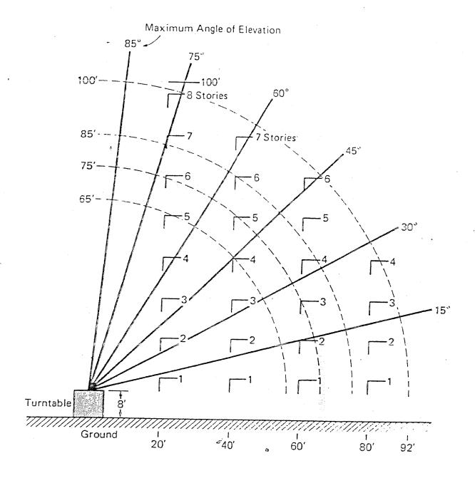
Approximate reach of aerial ladders at various lengths and angles. Sketch indicates average 12-foot heights between ceiling and floor levels. For example, at a 45 degree inclination an 85-foot ladder will reach the roof of an average five-story building but the 65-foot ladder barely tops a four-story building.
